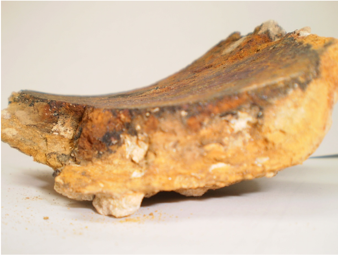
Figure 3.4 Damaged Water Main
