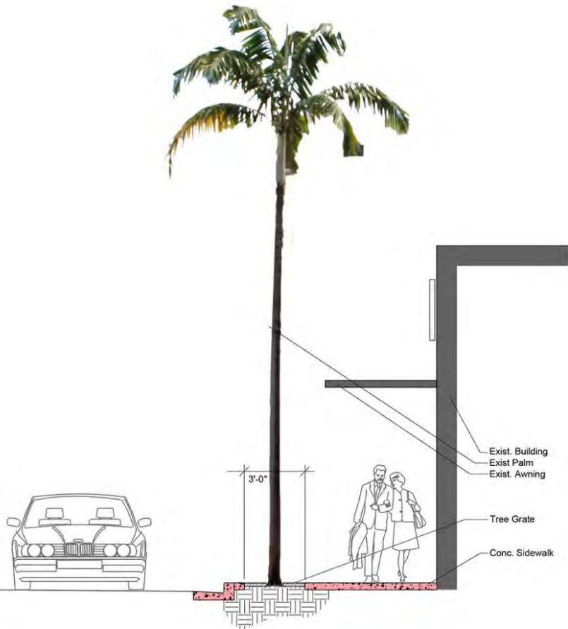
Existing Tree Planter Elevation
