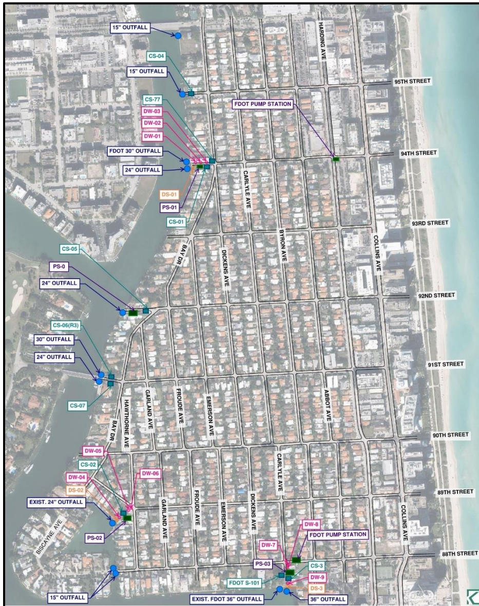
Figure 3 – Existing Stormwater Management System
