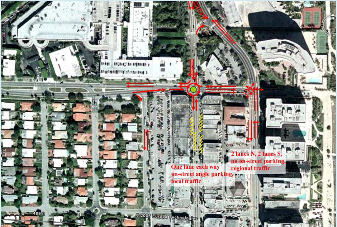
Figure 4: One-way to Two-way Operations Conversion
