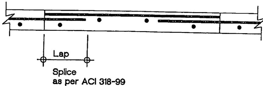
FOR REBAR DETERIORATED > 15%
