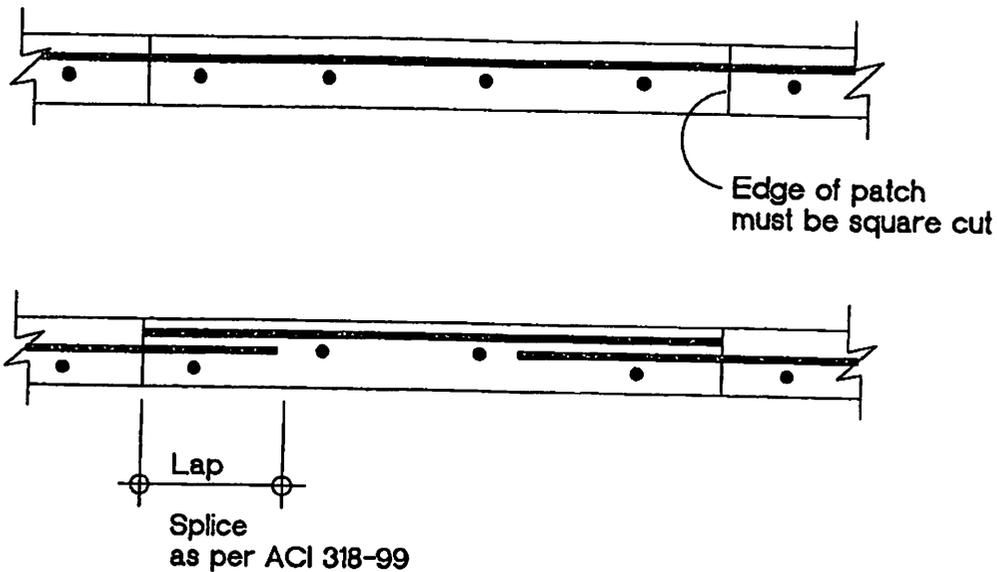
FOR REBAR DETERIORATED > 15%
