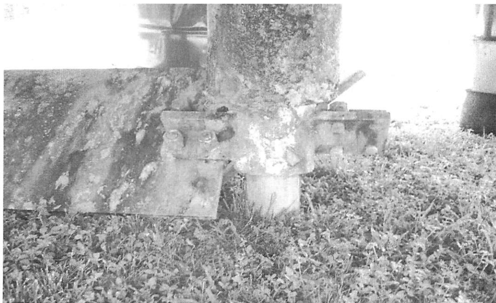
Oxygen Mixer with Broken Off Blades
