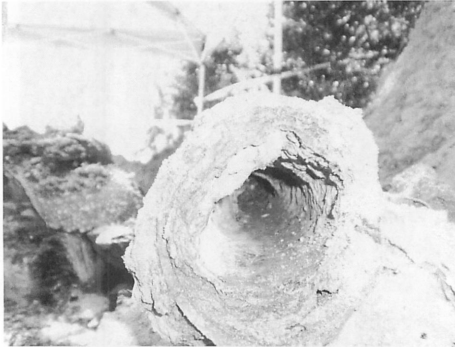
Figure 4.7 Example of Old Cast Iron Service Line in Very Deteriorated Condition – Exposed to Salt Water
