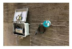
Figure 3. Installation of seismograph (at right) and monitoring data logger (at left) in progress at foundation wall of existing building.
