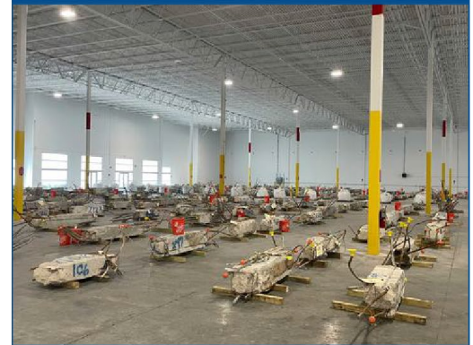
Concrete column evidence ready for material and structural testing (May 2023)
