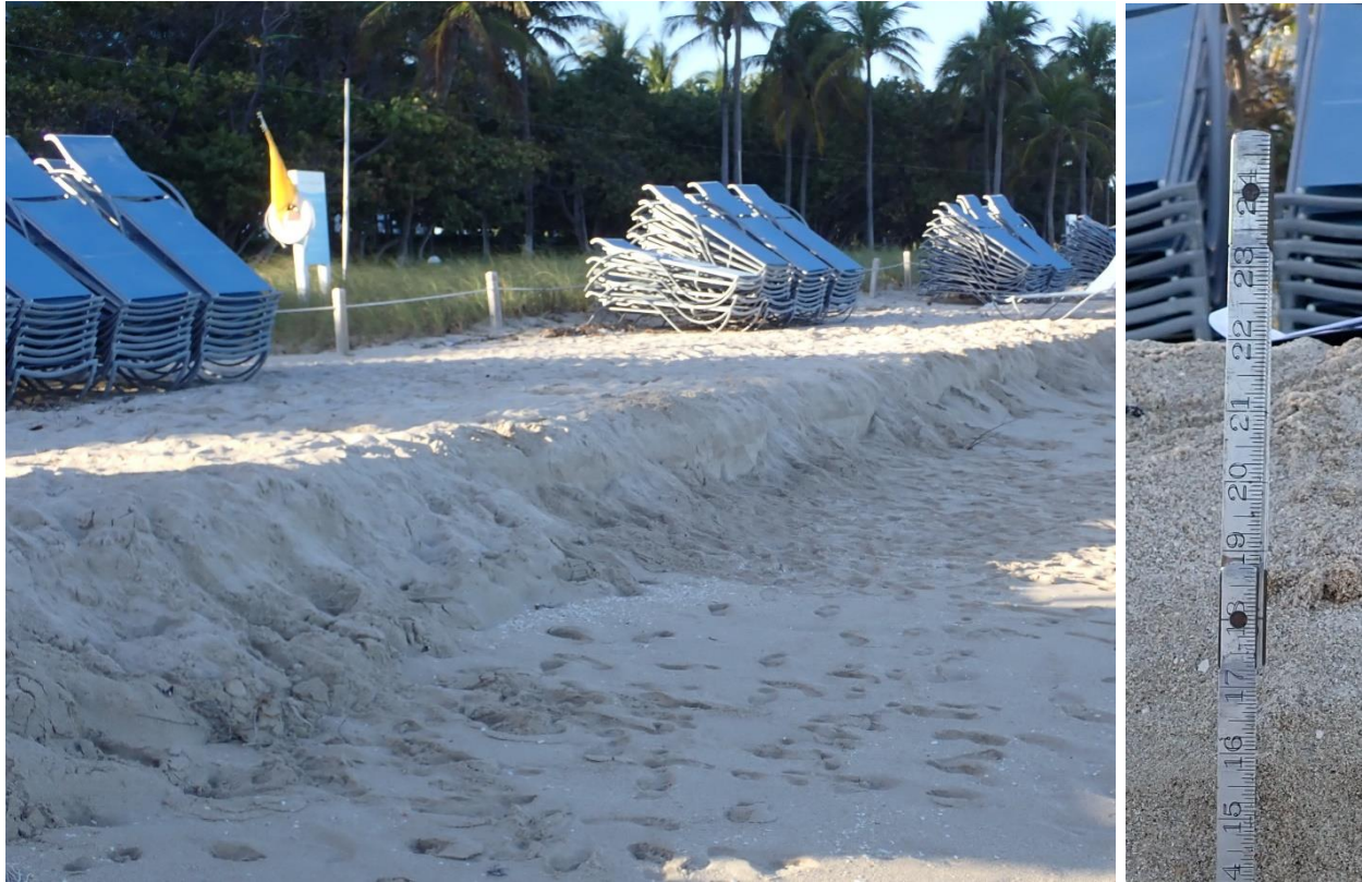
PHOTO 20. BEACH SCARP NORTH OF ACCESS 19, MEASURED 22 INCHES MAX
